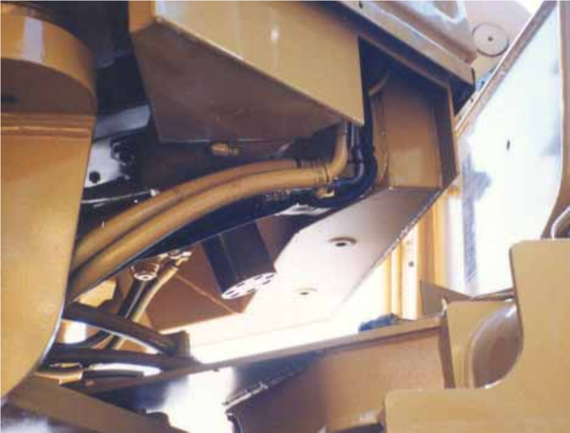
Underside of cab showing hoses to evaporator.
